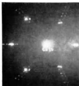
Fig.8. Laue photograph of crystal No. 3. Incident radiation makes an angle of 25^\circ 40' with the c axis; polytype 4H ; other conditions as in Fig.1.
