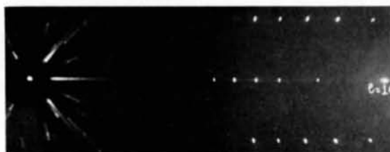
Fig. 2. a -axis 15^\circ -oscillation photograph of crystal No. 1; the angle between incident beam and c axis varies between 25^\circ and 40^\circ ; Cu K\alpha radiation; camera radius 3 cm; polytype 4H .
